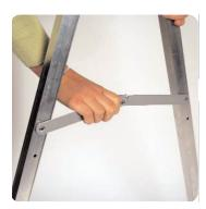
**STEP 2** Push each locking arm down to secure the frame
