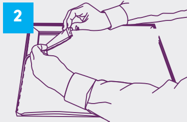
Start by pushing silicone bead into frame at corners
